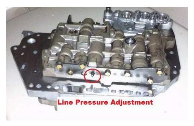
Reducing pressure adjustment is on the bottom side of the valvebody. It should be set to a minimum of line pressure divided by 2.35.
